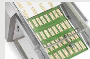
Electrical panning with pan movement for double discharge products. Programmable speed and product discharge
