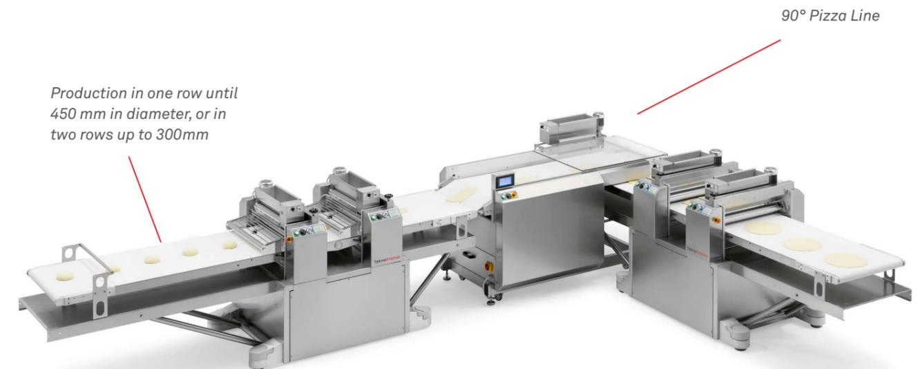
*Production in one row until 450 mm in diameter, or in two rows up to 300mm*
