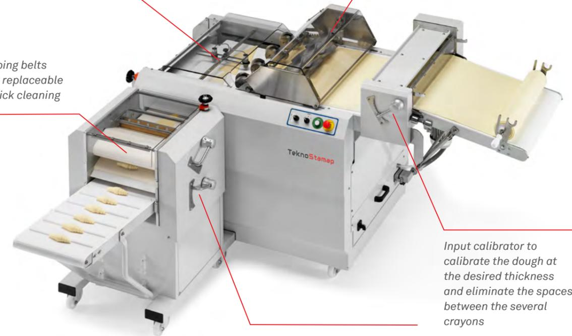
Input calibrator to calibrate the dough at the desired thickness and eliminate the spaces between the several croissants
